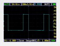
The J1772 Pilot is a 1khz +12V to -12V square wave, the voltage defines the state. The EV adds resistance pilot to Ground to vary the voltage. The EVSE reads the voltage and changes state accordingly.
