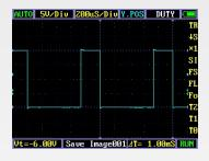
The J1772 Pilot is a 1khz +12V to -12V square wave, the Duty cycle (ratio high state to low state) determined the maximum available current. The EVSE sets the duty cycle the EV must comply to original setting or changes to the duty cycle.
