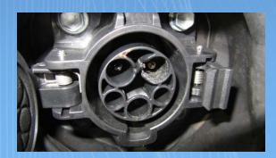
Newer EVs capable of drawing higher current are causing problems for even UL listed commercial EVSEs running at or below their rated limit.
